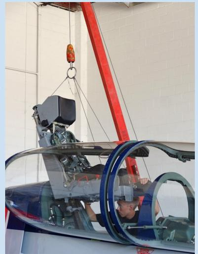
We can readily upgrade, install, and maintain hot seats. The FAA allows aircraft owners to have ejection seats, as long as they are maintained to a set of standards that are similar to the way the military used to maintain them. The seats require a yearly condition inspection, performed at the same time as the aircraft's inspection.
